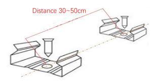
4.2. After installing the buckles, install the non-luminous side of the lamp into the buckle, and pull it to ensure that it will not fall off. Please see the picture below:
